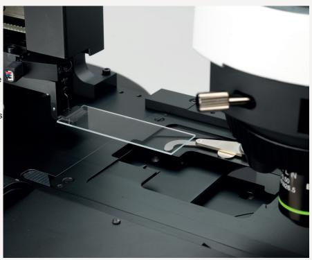
intentionally or unintentionally - the system responds by adjusting the height of the slide loading position accordingly. The presence of this height sensor also allows the system to work seamlessly with advanced auto-focus routines to maintain proper focus throughout the imaging cycle.
